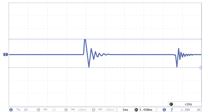
Figure 6 (d). Oscillograph chart of voltage transient deviation during load “drop/rise”.
