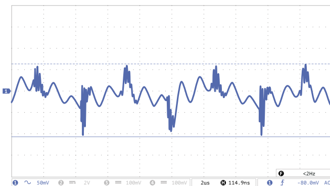
Figure 8 (c). Oscilloscope chart of output voltage ripple.
