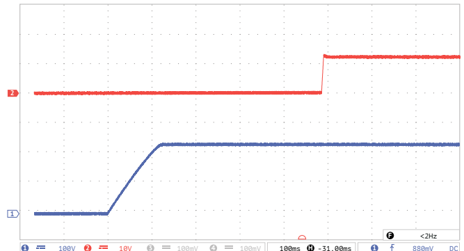
Figure 8 (b). Oscilloscope chart of output voltage after supplying the input voltage.
