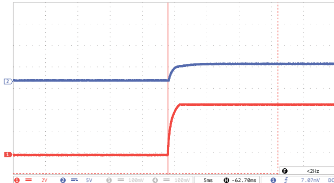
Figure 8 (a). Oscilloscope chart of setting output voltage after supplying remote control signal to ON-output.
