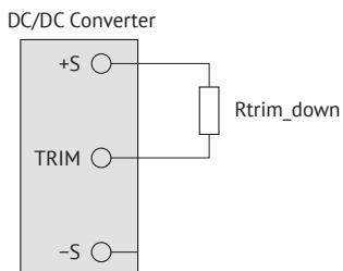
Figure 4. Resistor connection for U<sub>OUT,NOM</sub> trim down.
