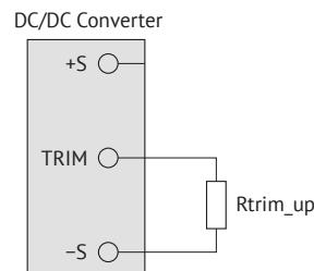
Figure 5. Resistor connection for U<sub>OUT,NOM</sub> trim up.
