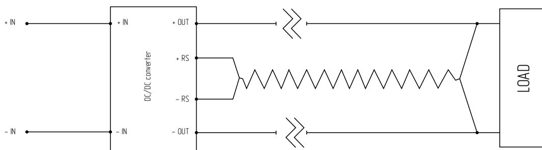
Figure 12. Typical connection diagram of external feedback application.
