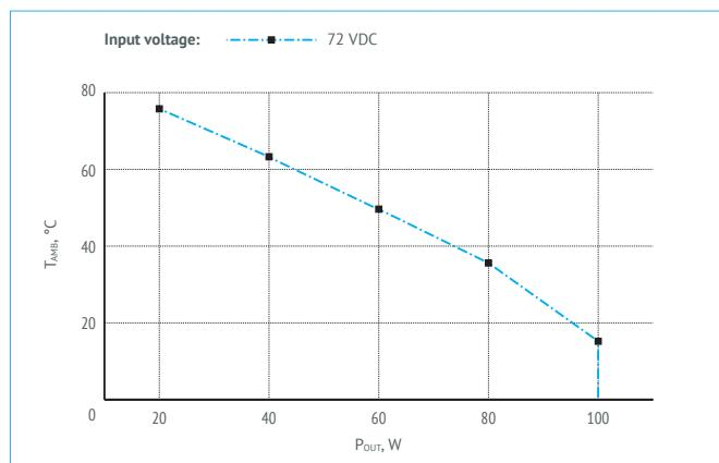
Figure 19. P<sub>OUT</sub> vs T<sub>AMB</sub> chart.
