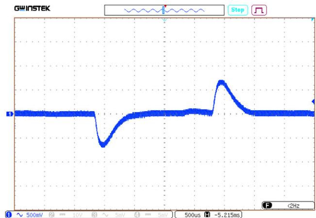
Figure 30.  $U_{OUT,NOM}$  transient deviation on  $0,75\dots 1 \times I_{OUT}$  change.
