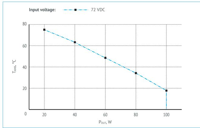
Figure 21. P<sub>OUT</sub> vs T<sub>AMB</sub> chart.
