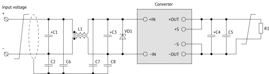
Figure 3. VDRW100 connection circuit for EN55032 Class B..
