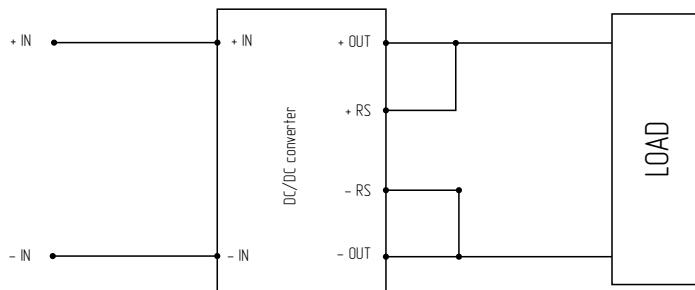
Figure 13. Typical connection diagram without external feedback application.
