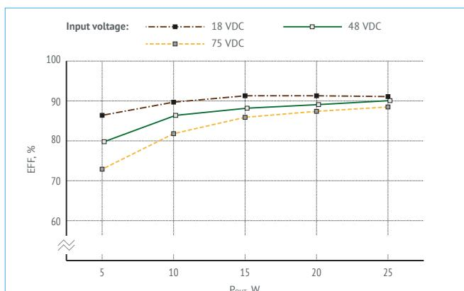
Figure 21. Efficiency of VDR125W12.
