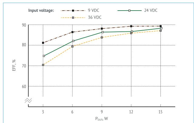
Figure 9. Efficiency of VDRI15B12.
