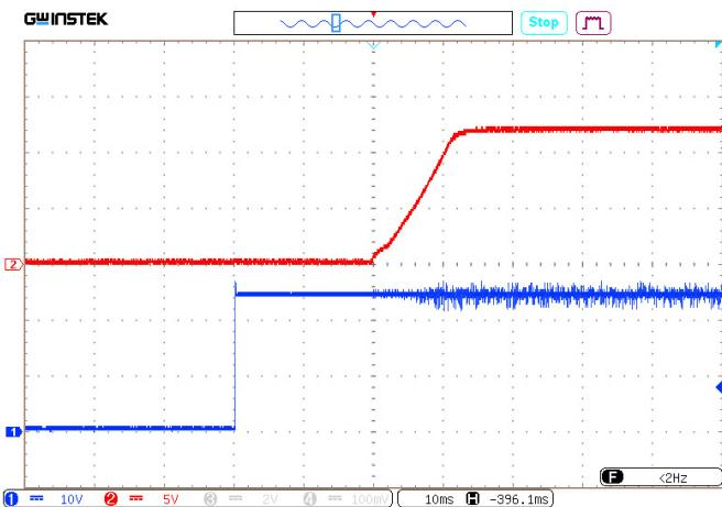
Figure 40.  $U_{OUT,NOM}$  stabilizing with  $U_{IN,NOM}$ .
