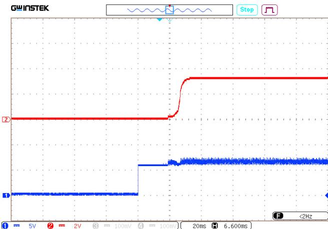
Figure 42.  $U_{OUT,NOM}$  stabilizing with Remote On/Off option (ON and -OUT pins connection).
