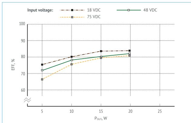
Figure 19. Efficiency of VDR125W3,3.
