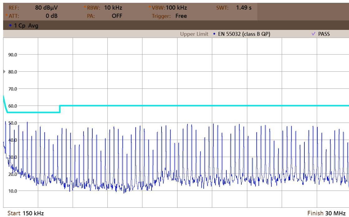
Figure 49. Compliance spectrogram EN55032 Class B (0,15–30 MHz).
