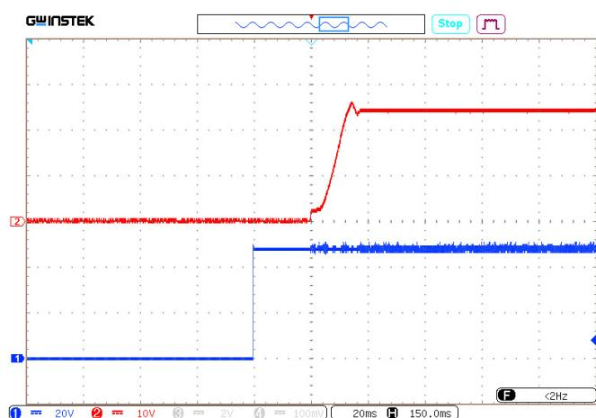
Figure 36.  $U_{OUT,NOM}$  stabilizing with  $U_{IN,NOM}$ .
