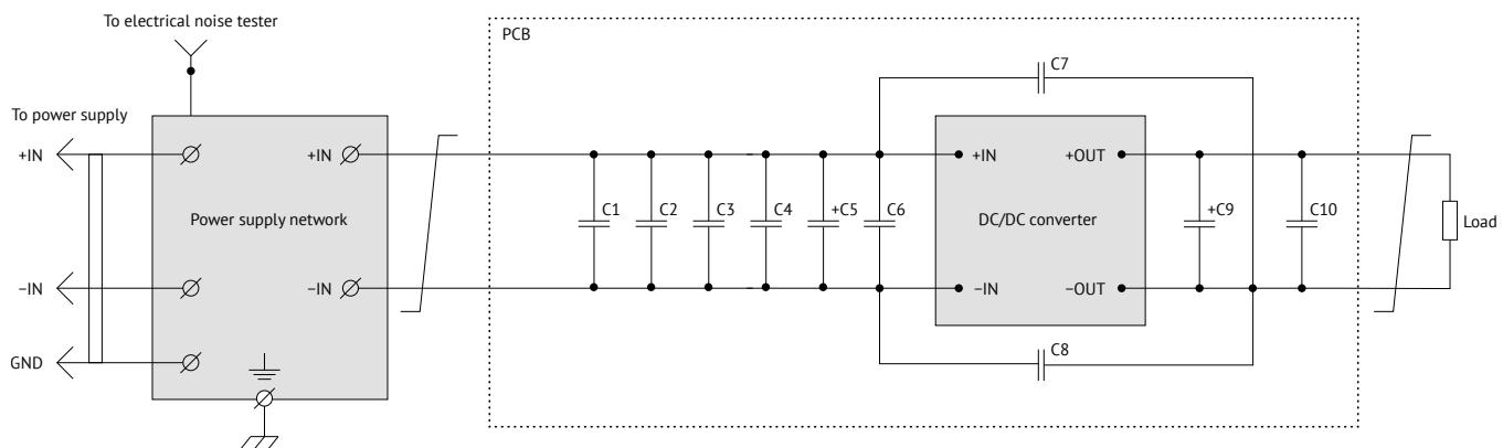
Figure 3. Connection diagram VDR115, VDR125.
