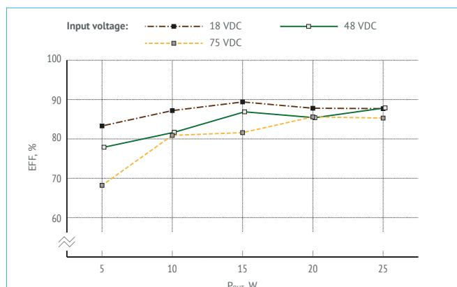
Figure 22. Efficiency of VDR125W24.
