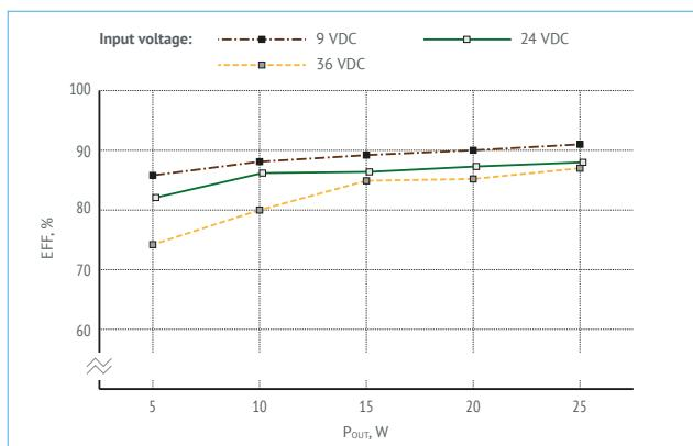
Figure 17. Efficiency of VDR125B24.
