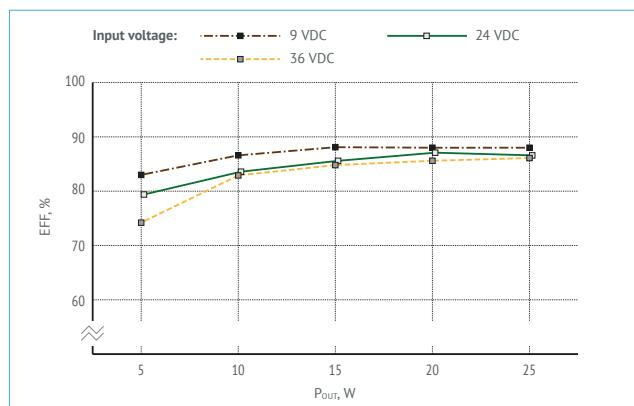
Figure 18. Efficiency of VDR125B48.
