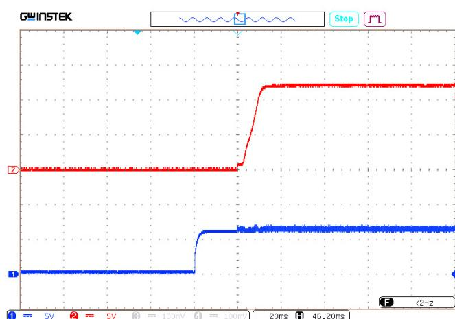
Figure 38.  $U_{OUT,NOM}$  stabilizing with Remote On/Off option (ON and -OUT pins connection).
