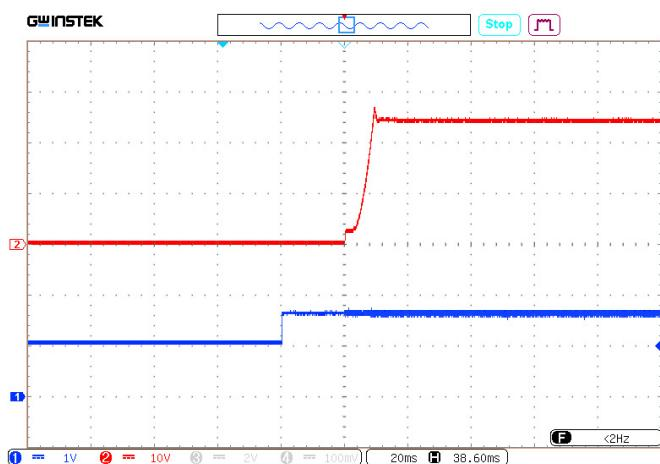
Figure 35.  $U_{OUT,NOM}$  stabilizing with Remote On/Off option (control signal).
