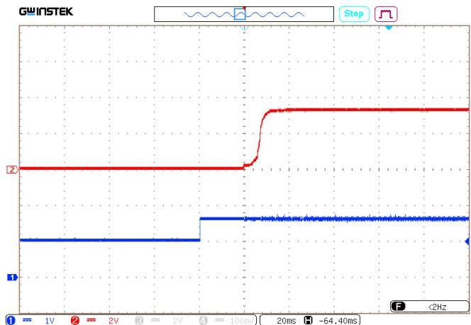
Figure 43.  $U_{OUT,NOM}$  stabilizing with Remote On/Off option (control signal).
