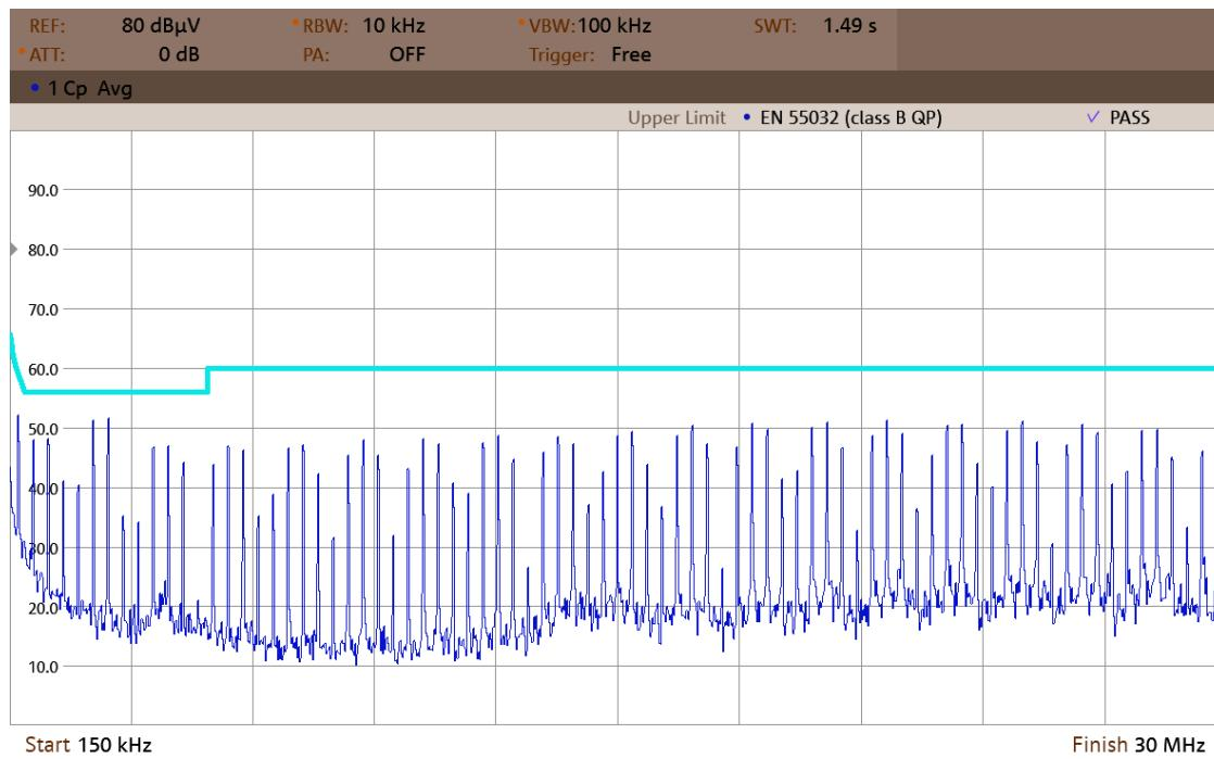
Figure 53. Compliance spectrogram EN55032 Class B (0,15–30 MHz).
