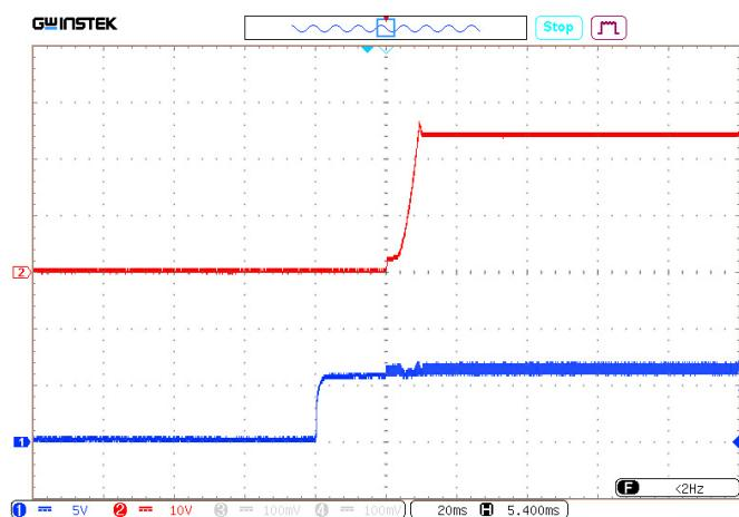
Figure 34.  $U_{OUT,NOM}$  stabilizing with Remote On/Off option (ON and -OUT pins connection).
