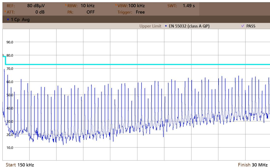
Figure 50. Compliance spectrogram EN55032 Class A (0,15–30 MHz).
