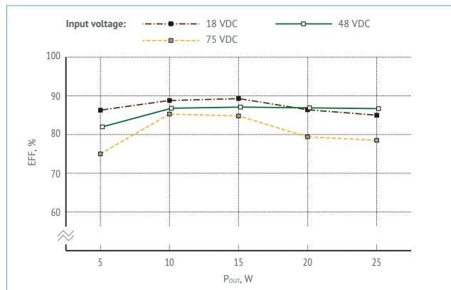
Figure 20. Efficiency of VDR125W05.
