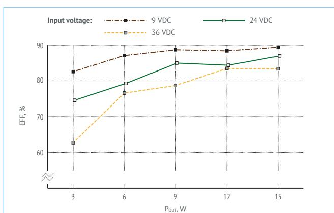
Figure 10. Efficiency of VDRI15B24.
