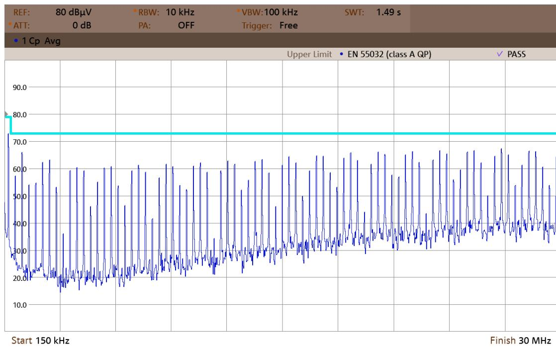
Figure 52. Compliance spectrogram EN55032 Class A (0,15–30 MHz).
