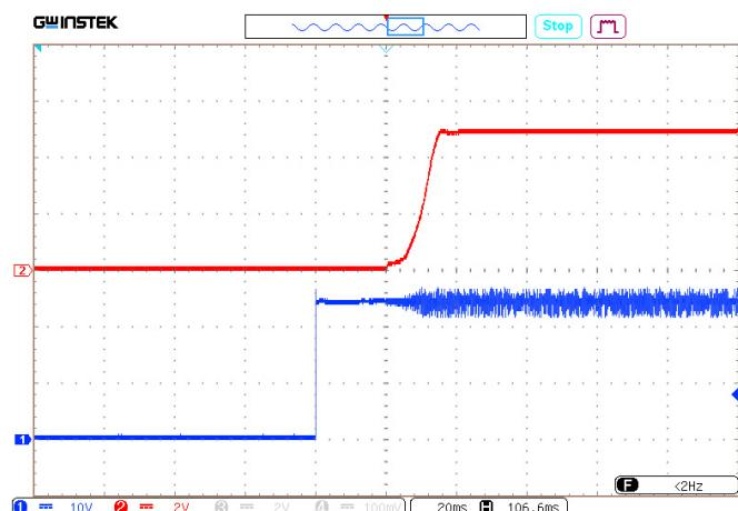
Figure 32.  $U_{OUT,NOM}$  stabilizing with  $U_{IN,NOM}$ .
