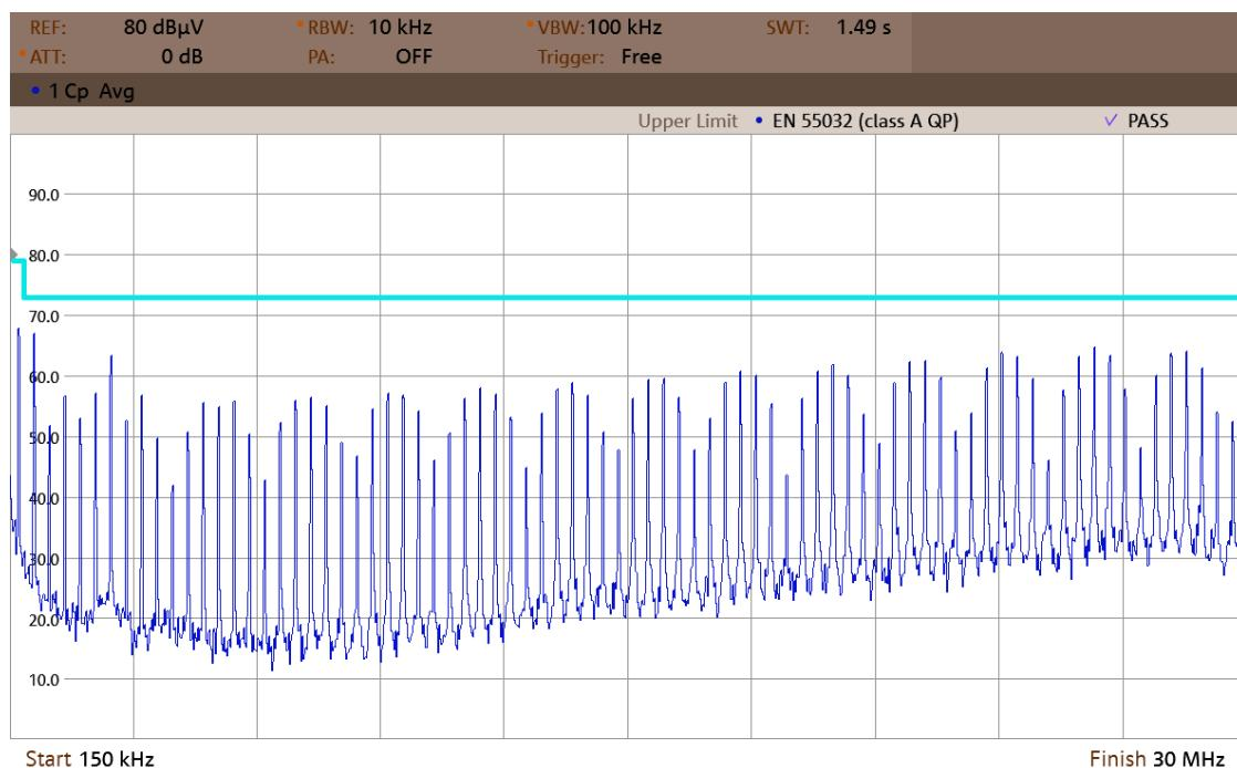
Figure 46. Compliance spectrogram EN55032 Class A (0,15–30 MHz).
