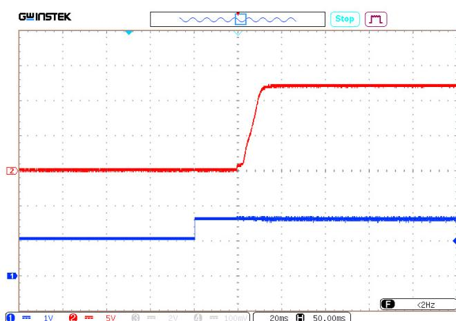
Figure 39.  $U_{OUT,NOM}$  stabilizing with Remote On/Off option (control signal).
