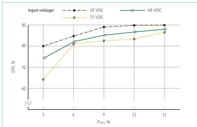
Figure 14. Efficiency of VDRI15W48.
