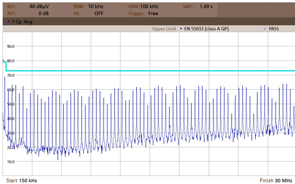
Figure 48. Compliance spectrogram EN55032 Class A (0,15–30 MHz).
