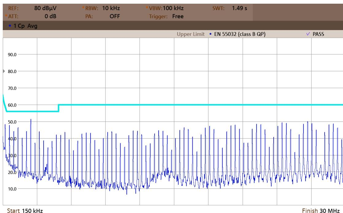
Figure 47. Compliance spectrogram EN55032 Class B (0,15–30 MHz).
