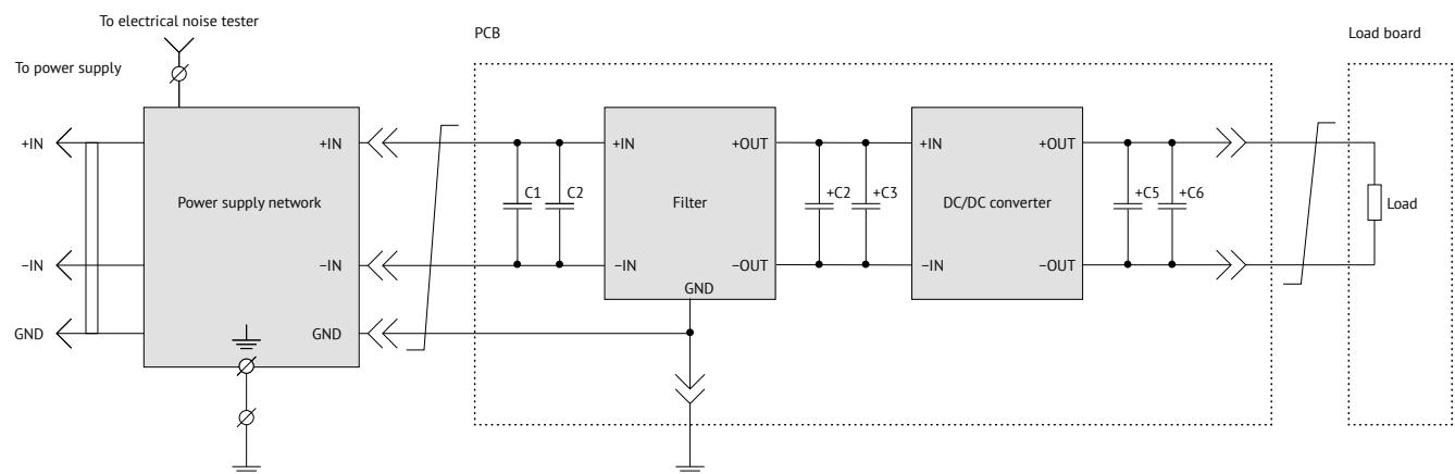
Figure 5. Connection diagram VDR115, VDR125.
