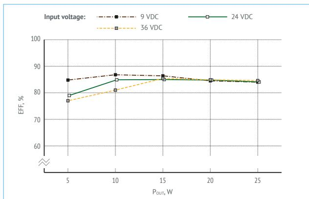
Figure 15. Efficiency of VDRI25B05.
