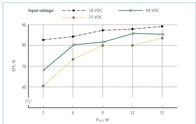
Figure 13. Efficiency of VDRI15W24.
