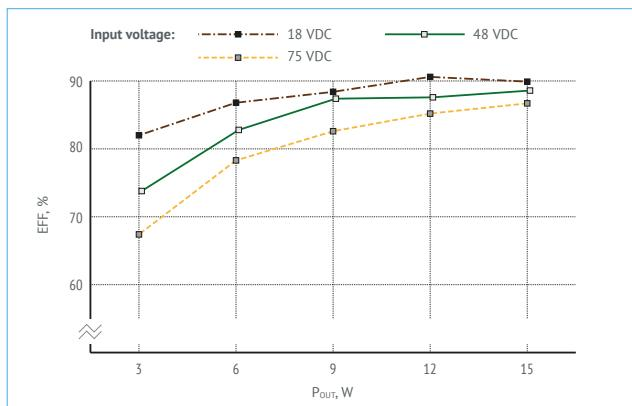
Figure 12. Efficiency of VDRI15W12.
