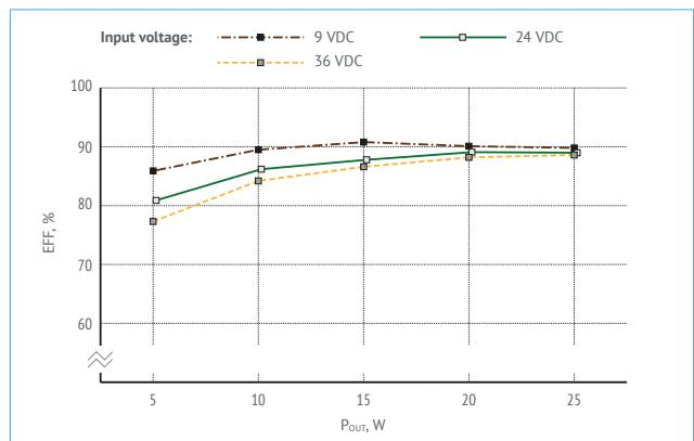
Figure 16. Efficiency of VDRI25B12.
