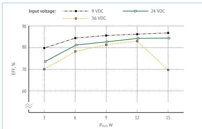
Figure 8. Efficiency of VDRI15B05.
