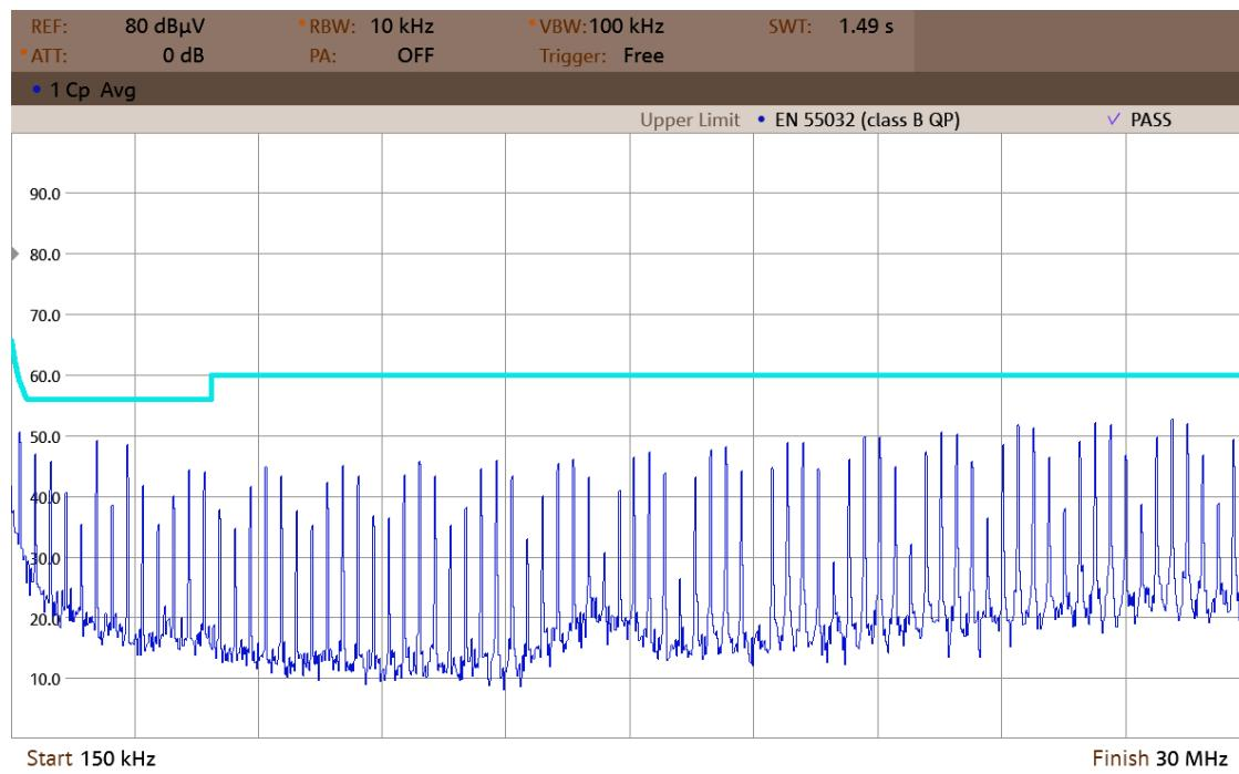
Figure 51. Compliance spectrogram EN55032 Class B (0,15–30 MHz).
