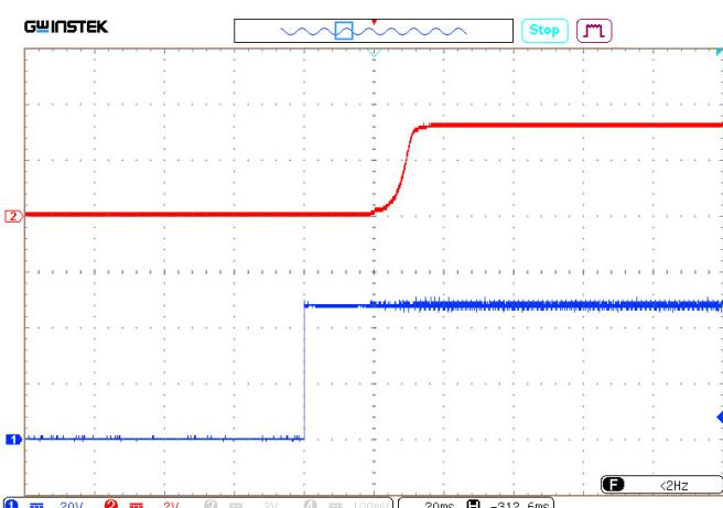
Figure 44.  $U_{OUT,NOM}$  stabilizing with  $U_{IN,NOM}$ .
