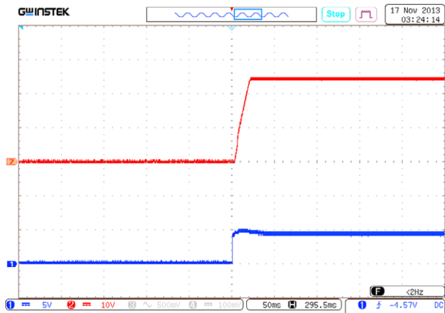
Figure 10 (a). Oscilloscope chart of setting output voltage after supplying remote control signal to ON-input.
