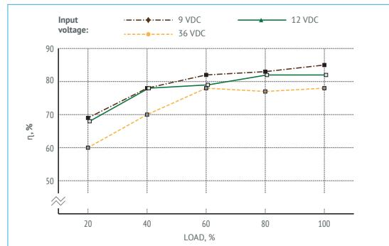
Figure 7 (a). Efficiency of VDR15B3.3.
