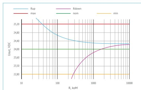
Figure 5 (f). Resistance values for adjustment of  $U_{out}=24$  VDC.
