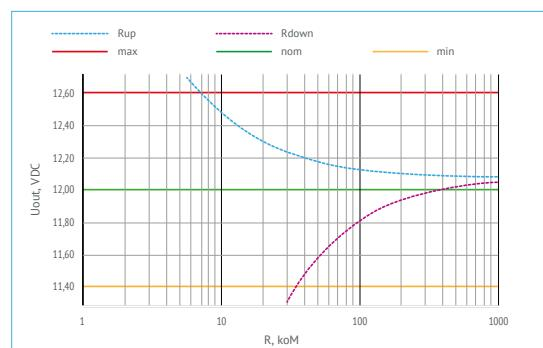
Figure 5 (d). Resistance values for adjustment of  $U_{out}=12$  VDC.
