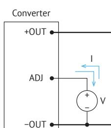
Figure 4 (d). Adjustment by voltage source.
