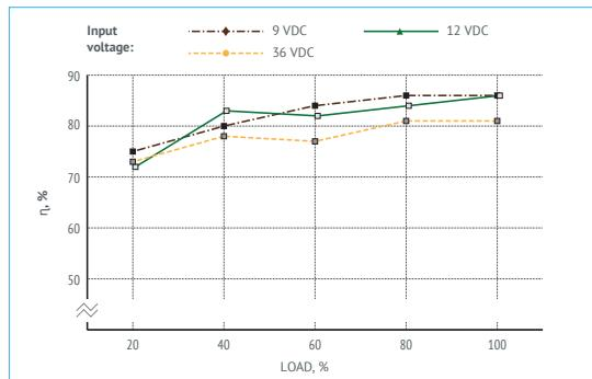
Figure 7 (f). Efficiency of VDR15B24.
