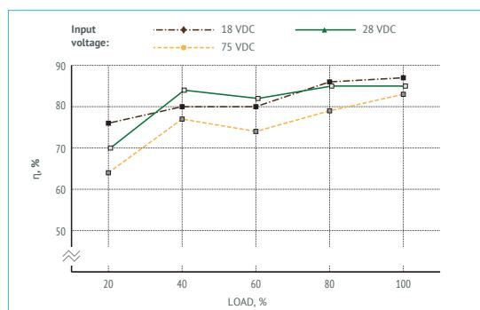
Figure 8 (f). Efficiency of VDR15W24.
