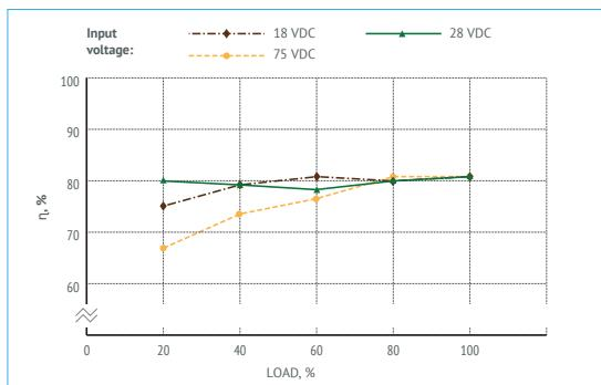
Figure 9 (c). Efficiency of VDR25W05.
