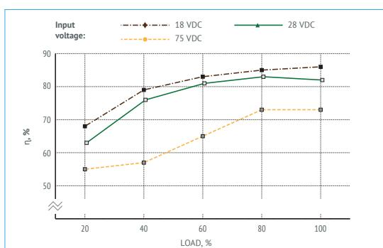
Figure 8 (c). Efficiency of VDR15W09.
