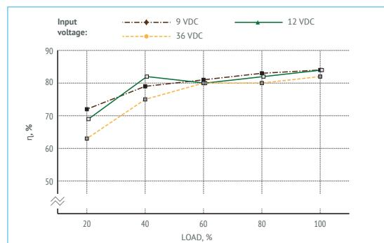
Figure 7 (g). Efficiency of VDR15B28.
