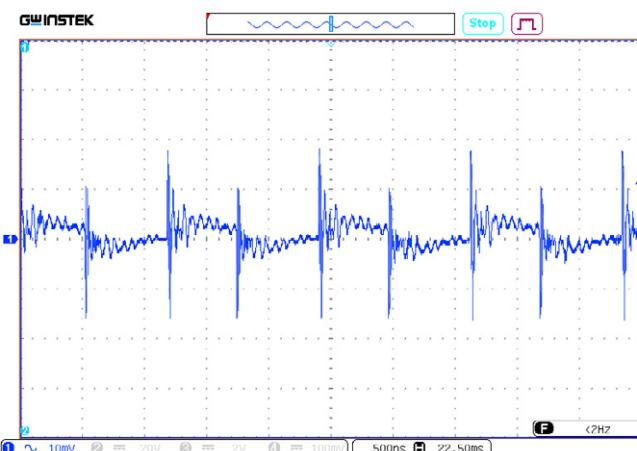
**Figure 10 (c).** Oscillograph chart of output voltage ripple.
