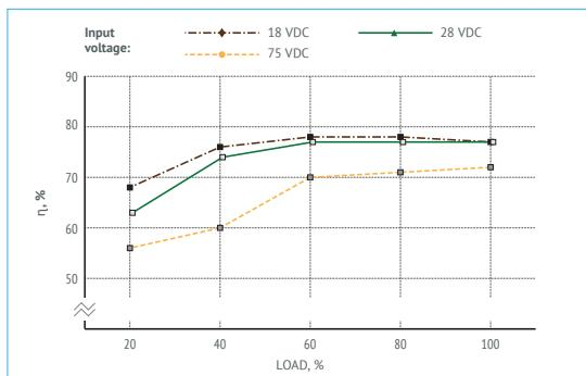
Figure 8 (a). Efficiency of VDR15W3.3.
