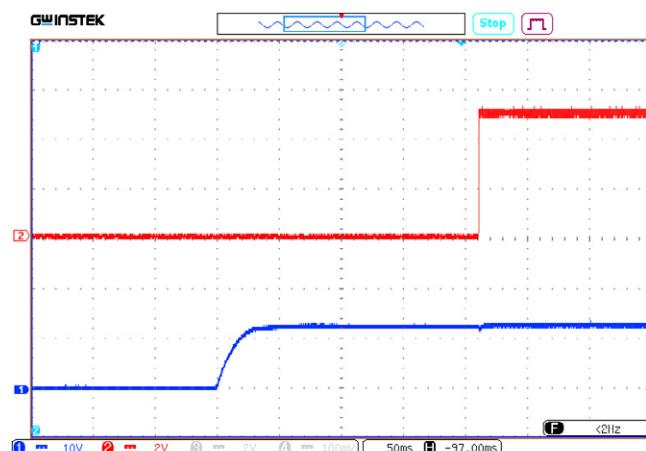
**Figure 10 (b).** Oscillograph chart of output voltage after supplying the input voltage.
