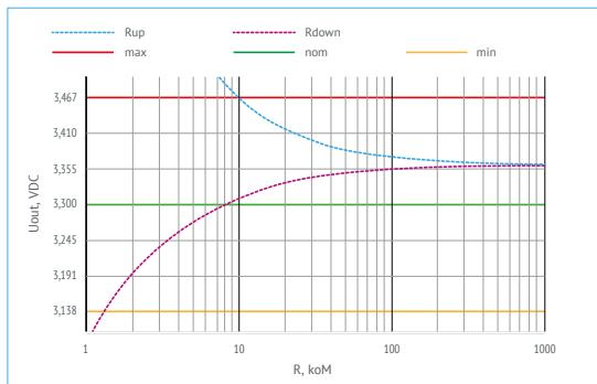
Figure 5 (a). Resistance values for adjustment of  $U_{out}=3.3$  VDC.
