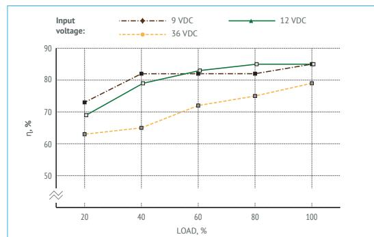
Figure 7 (c). Efficiency of VDR15B09.
