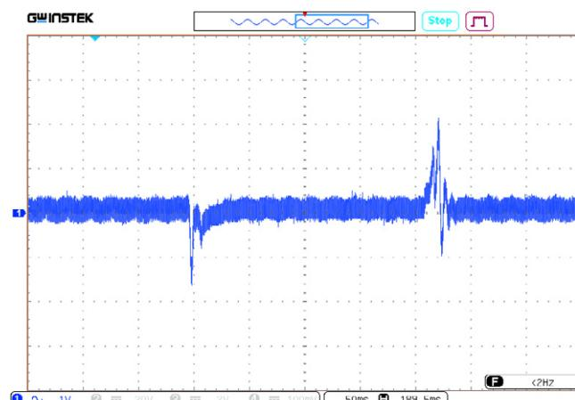
**Figure 11 (d).** Oscillograph chart of voltage transient deviation during load “drop/rise” 0...100 %.
