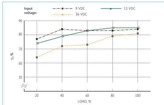
Figure 7 (b). Efficiency of VDR15B05.
