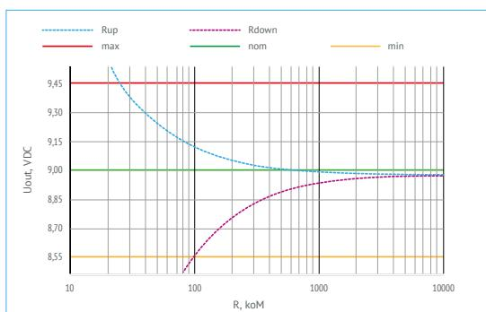
Figure 5 (c). Resistance values for adjustment of  $U_{out}=9$  VDC.
