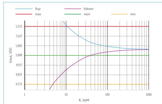
Figure 5 (b). Resistance values for adjustment of  $U_{out}=5$  VDC.
