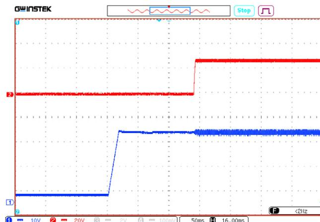
**Figure 11 (b).** Oscillograph chart of output voltage after supplying the input voltage.
