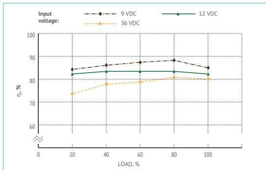
Figure 9 (a). Efficiency of VDR25B05.
