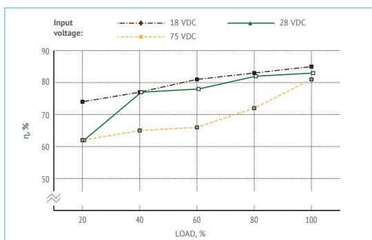
Figure 8 (e). Efficiency of VDR15W15.
