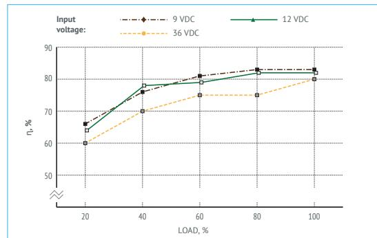
Figure 7 (e). Efficiency of VDR15B15.
