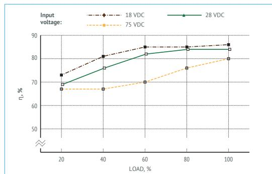
Figure 8 (b). Efficiency of VDR15W05.
