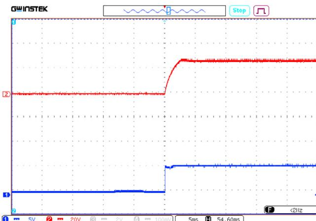
**Figure 11 (a).** Oscillograph chart of setting output voltage after supplying remote control signal to ON-input.
