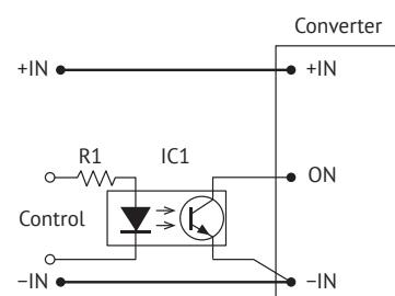
Figure 3 (c). ON/OFF control by optocoupler.
