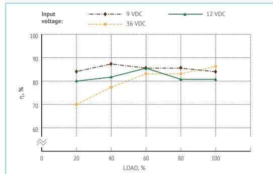
Figure 9 (b). Efficiency of VDR25B24.
