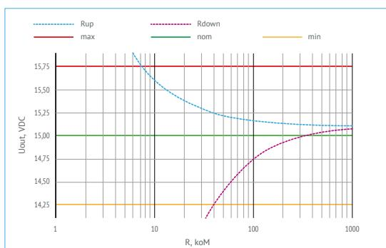
Figure 5 (e). Resistance values for adjustment of  $U_{out}=15$  VDC.
