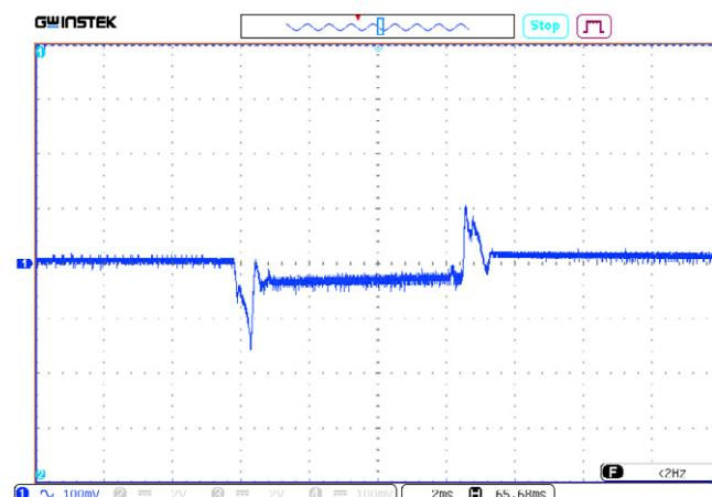
**Figure 10 (d).** Oscillograph chart of voltage transient deviation during load "drop/rise" 0...100 %.
