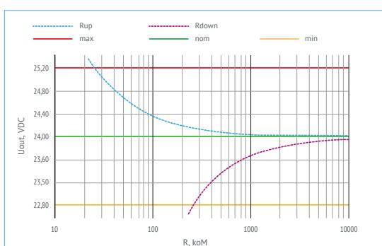
Figure 5 (g). Current and voltage values for adjustment of VDR160[...]24.
