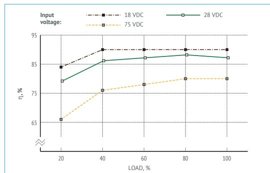
Figure 7 (b). Efficiency of VDR160W09.
