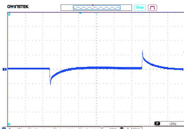
**Figure 9 (d).** Oscillograph chart of voltage transient deviation during load "drop/rise" 0...100 %.
