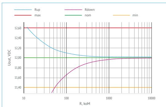
Figure 5 (e). Current and voltage values for adjustment of VDR160[...]12.
