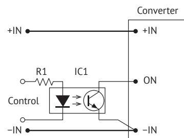
Figure 3 (c). ON/OFF control by optocoupler.
