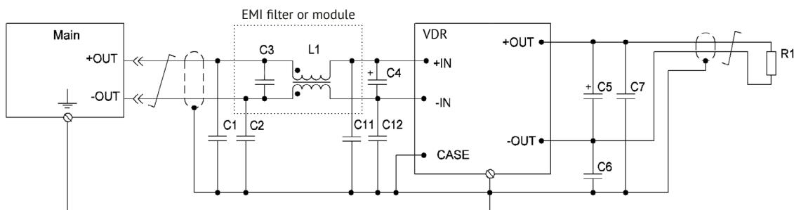
Figure 2. Typical connection with filtration unit.
