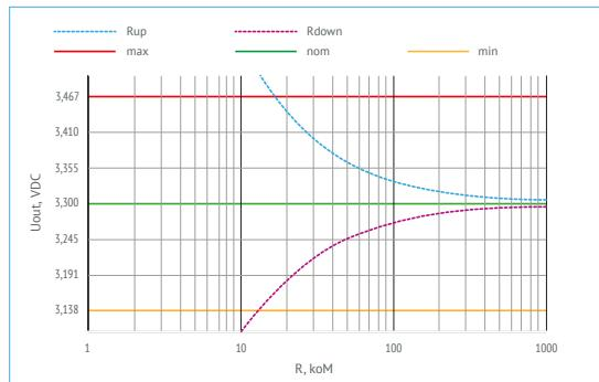
Figure 5 (b). Current and voltage values for adjustment of VDR120W3.3.
