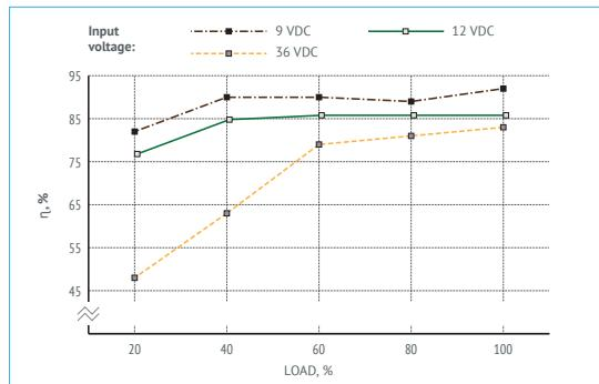
Figure 6 (b). Efficiency of VDR160B09.
