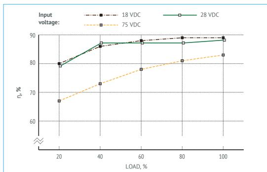
Figure 7 (e). Efficiency of VDR160W28.
