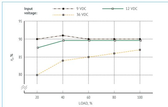
Figure 6 (a). Efficiency of VDR160B05.
