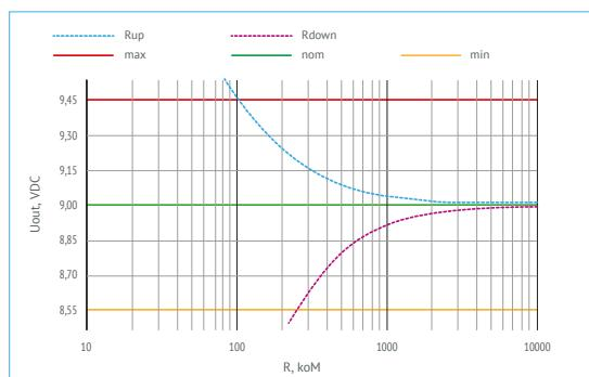
Figure 5 (d). Current and voltage values for adjustment of VDR160[...]09.
