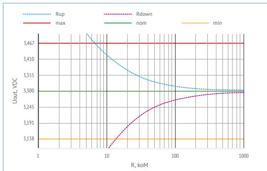
Figure 5 (a). Current and voltage values for adjustment of VDR120B3.3.
