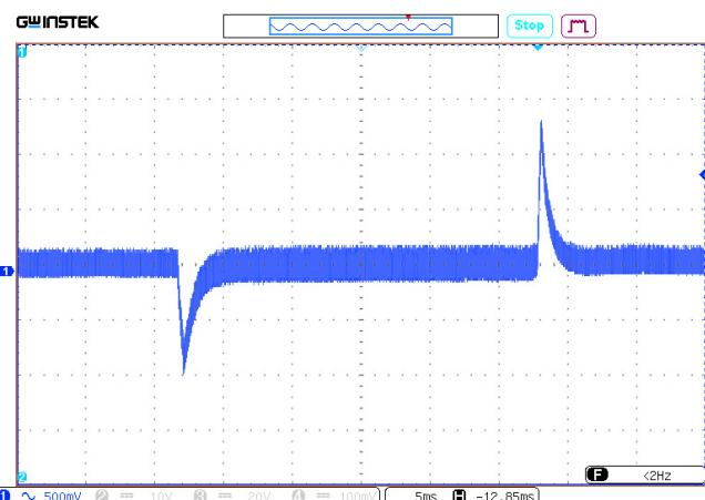
**Figure 8 (d).** Oscillograph chart of voltage transient deviation during load "drop/rise" 0...100 %.
