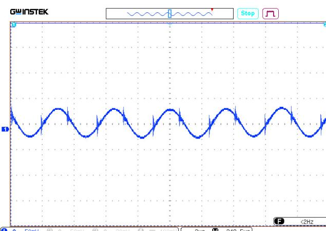
**Figure 9 (c).** Oscillograph chart of output voltage ripple.
