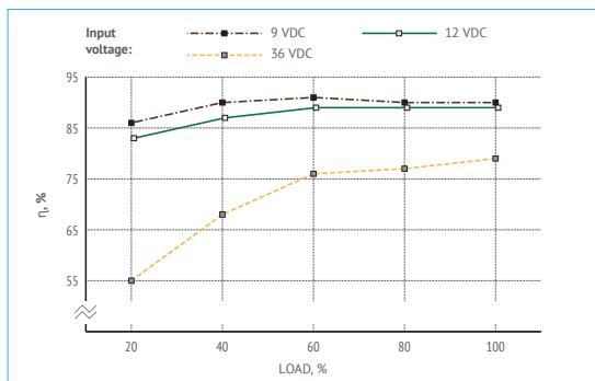
Figure 6 (c). Efficiency of VDR160B12.
