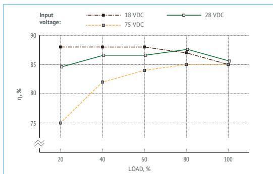
Figure 7 (a). Efficiency of VDR160W05.
