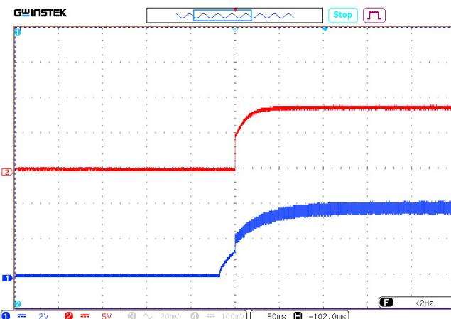
**Figure 9 (a).** Oscillograph chart of setting output voltage after supplying remote control signal to ON-input.
