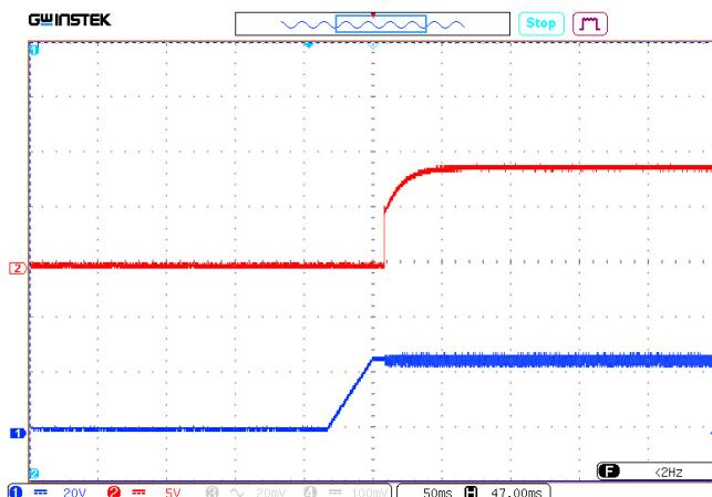
**Figure 9 (b).** Oscillograph chart of output voltage after supplying the input voltage.
