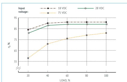
Figure 7 (c). Efficiency of VDR160W12.
