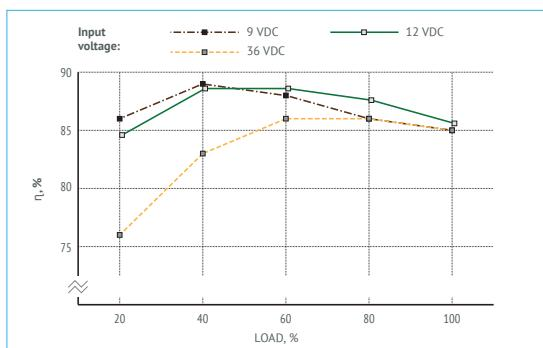
Figure 6 (a). Efficiency of VDR100B05.
