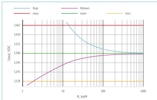
Figure 5 (a). Output voltage and resistor rating of  $U_{out}=3,3$  VDC.
