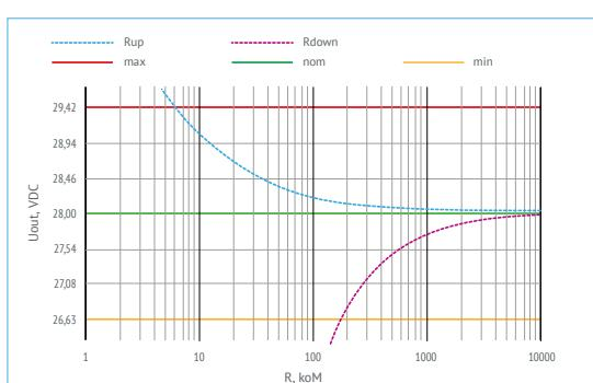
Figure 5 (g). Output voltage and resistor rating of  $U_{out}=28$  VDC.
