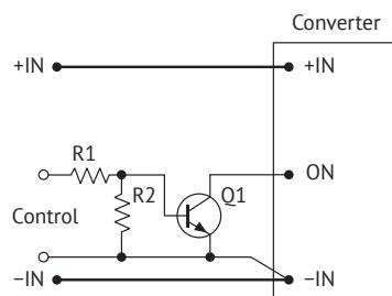
Figure 3 (b). ON/OFF control by bipolar transistor.
