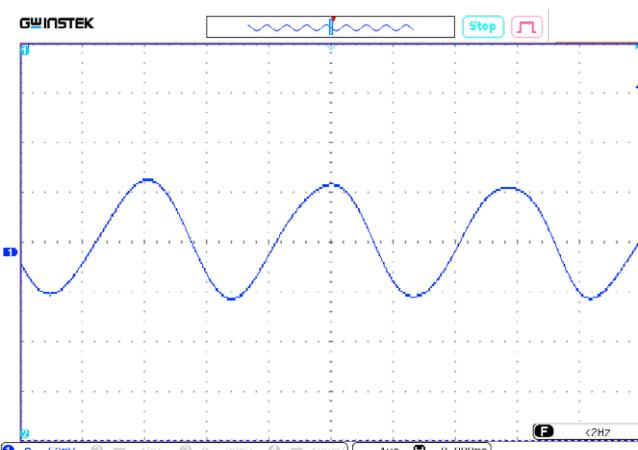
**Figure 8 (c).** Oscillograph chart of output voltage ripple.
