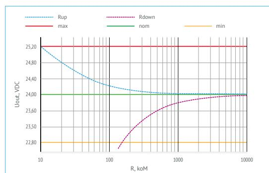
Figure 5 (f). Output voltage and resistor rating of  $U_{out}=24$  VDC.
