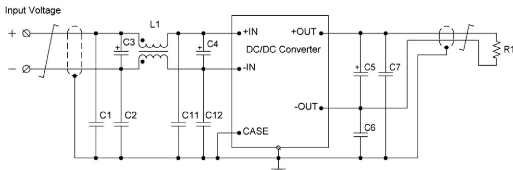
**Figure 2.** Typical connection with filtration unit for VDR75 and VDR100.
