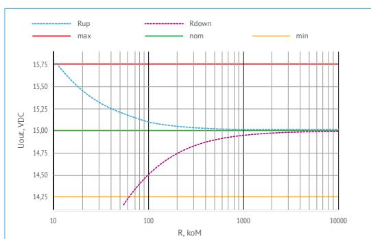
Figure 5 (e). Output voltage and resistor rating of  $U_{out}=15$  VDC.
