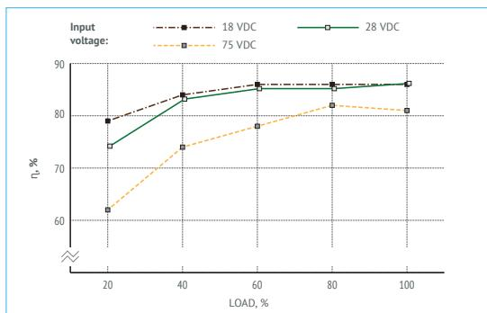
Figure 7 (e). Efficiency of VDR100W28.
