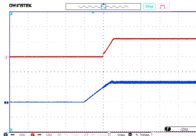
**Figure 8 (b).** Oscillograph chart of output voltage after supplying the input voltage.
