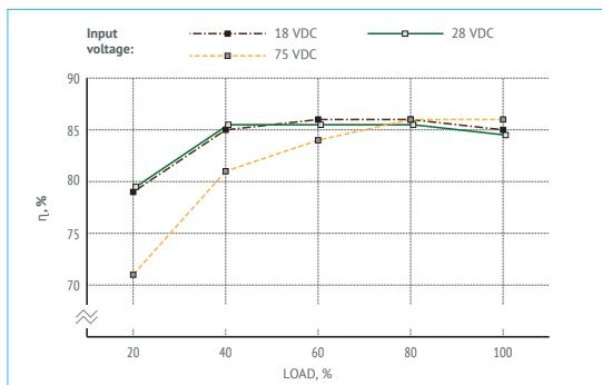
Figure 7 (a). Efficiency of VDR100W05.
