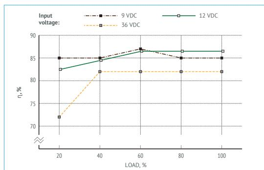
Figure 6 (b). Efficiency of VDR100B09.
