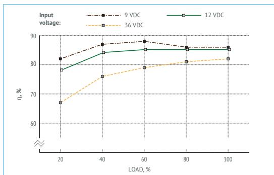
Figure 6 (e). Efficiency of VDR100B24.
