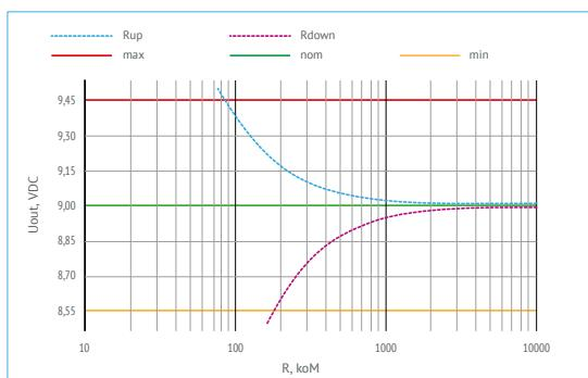
Figure 5 (c). Output voltage and resistor rating of  $U_{out}=9$  VDC.
