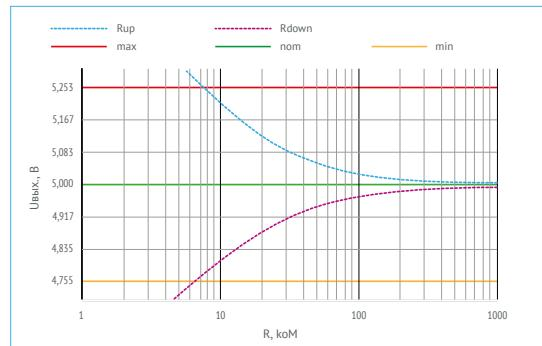
Figure 5 (b). Output voltage and resistor rating of  $U_{out}=5$  VDC.
