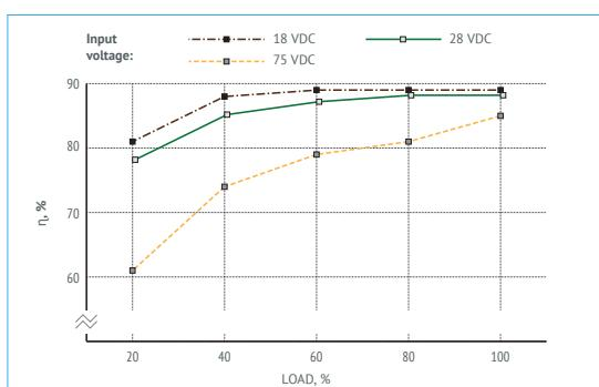
Figure 7 (c). Efficiency of VDR100W12.
