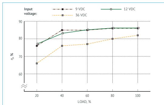
Figure 6 (f). Efficiency of VDR100B28.
