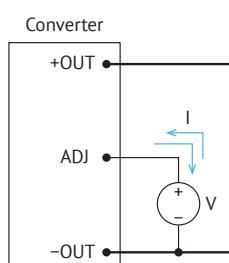
Figure 4 (d). Adjustment by voltage source.
