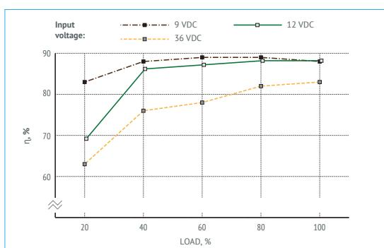
Figure 6 (c). Efficiency of VDR100B12.
