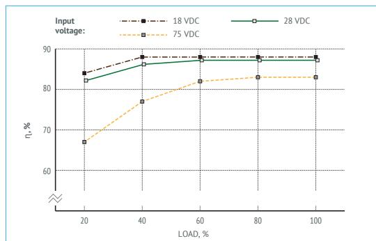
Figure 7 (b). Efficiency of VDR100W09.
