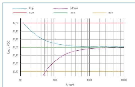
Figure 5 (d). Output voltage and resistor rating of  $U_{out}=12$  VDC.
