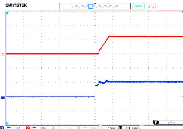
**Figure 8 (a).** Oscillograph chart of setting output voltage after supplying remote control signal to ON-input.
