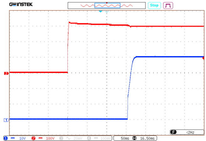
Figure 10 (b). Oscilloscope chart of output voltage after supplying the input voltage.
