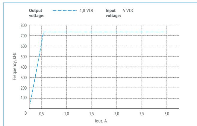
Pic. 5. The dependence of the conversion frequency on the load current.
