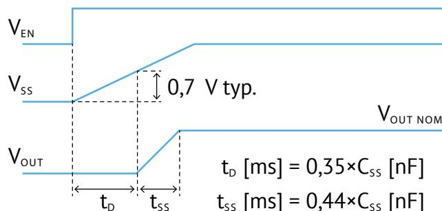
Pic. 20. Converter's "soft-start" diagram.
