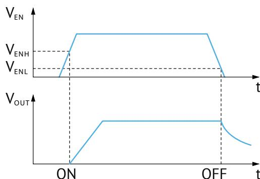
Pic. 14. ON/OFF depending on  $V_{EN}$ .
