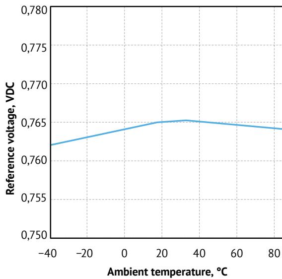
Pic. 19. Typical dependence of the reference voltage on temperature.  $V_{IN} = 12$  VDC.
