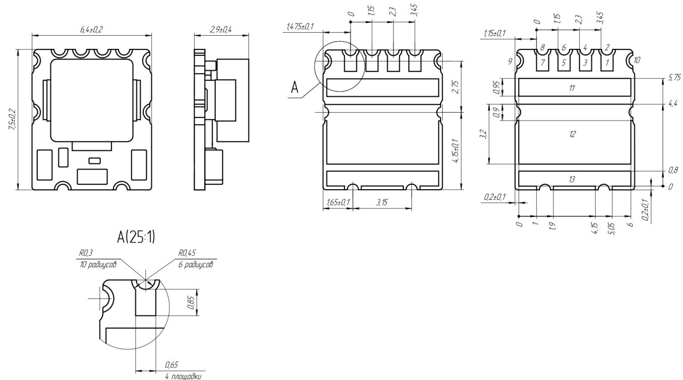
Pic. 21. When mounting, it is recommended to use all contact pads, especially PGND, as it is used for heat conduction.
