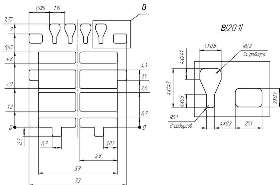
Pic. 25. Solder paste example based on 0.1 mm thick stencil.
