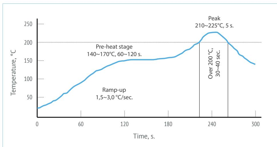
Pic. 26. Reflowing in a convection heating oven.
