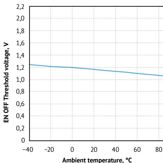
Pic. 18. Temperature dependence of  $V_{ENL}$  threshold.
