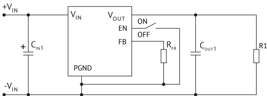
Pic. 30. Typical connection diagram for VNA3L0, 87, OSP.
