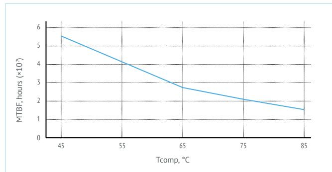
Pic. 4. MTBF vs. components temperature (T<sub>COMP</sub>) curve. MIL-STD-217F, group Gb.
