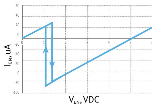
Pic. 16. Typical hysteresis of switching on / off the module on the EN output.
