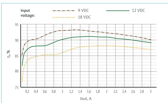
Pic. 11.  $V_{IN} = 9\ldots18\text{V}$ ;  $V_{OUT} = 5\text{V}$ .
