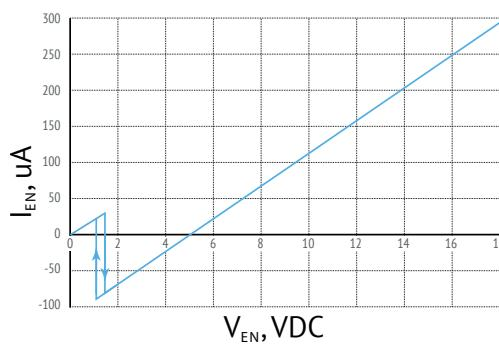
Pic. 15. A typical curve of the sinking/sourcing current on the EN pin, depending on the voltage on it.  $V_{IN} = 18 \text{ VDC}$ .
