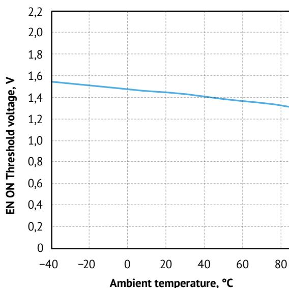
Pic. 17. Temperature dependence of  $V_{ENH}$  threshold.
