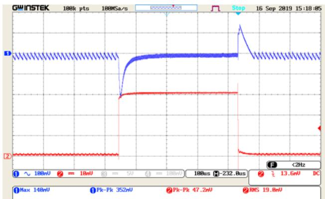
Pic. 7.  $I_{OUT} = 0,1\text{-}3 \text{ A}; 6,5 \text{ A}/\mu\text{s}$ .
